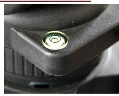
Bubble level as part of the tripod head
